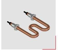
Tubular heaters are a safe and efficient heating option, using a resistive coil inside a metal tube filled with insulating magnesium oxide. This design prevents electric shock and transfers heat efficiently to the surface, making them ideal for modern heating needs.
